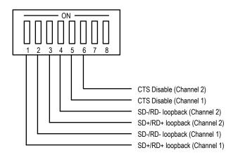
The Mode #2 switch controls the RS-485 loopback feature, connecting the SD+/- signals to the RD+/- signals internally so you don't have to make the connection on your cable. It also controls the CTS disable feature and the output of the clock in RS-485 mode. Since the 82532 will only transmit when its CTS pin is active, this switch allows the 82532 to see the CTS input as active all the time, regardless of the signal at the connector.
