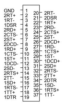
The cable provided splits each channel from this DB37 to individual RS-530 pin out DB25 male connectors. The DB25 pin outs are shown on the next page.
