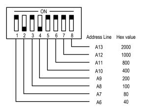
Address lines A6 through A13 are decoded by the setting of SW1 and set the base address of the FASTCOM™: ESCC-104. Address lines A0 - A5 are used on the board to select configuration and control registers on the 82532 chip.
