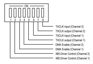
The Mode #1 switch serves three functions: it selects either RS-422 or RS-485 driver mode, enables or disables DMA, and selects the direction of the transmit clock (input or output).
