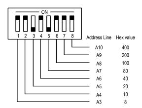
Address lines A5 through A12 are decoded by the setting of SW1 and set the address of each channel of the FASTCOM: 422/4-104-ET. Address lines A3 and A4 are used on the board to select which port (1, 2, 3, or 4) you want to use. Address lines A0, A1, and A2 are used to select the registers within the UARTs.
