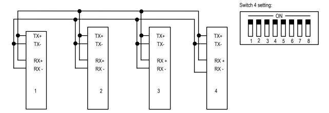
Note: The termination resistors from Station #2 and Station #3 have been removed.
