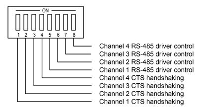
Switch positions 1, 2, 3, and 4 enable or disable CTS handshaking for each channel. When ON, CTS handshaking is disabled; when OFF, CTS handshaking is enabled. In RS-485 mode, CTS handshaking is usually disabled.
