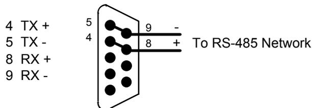
Note that when in the RS-485 mode, you will need to externally connect TX+ to RX+ and TX- to RX-.
