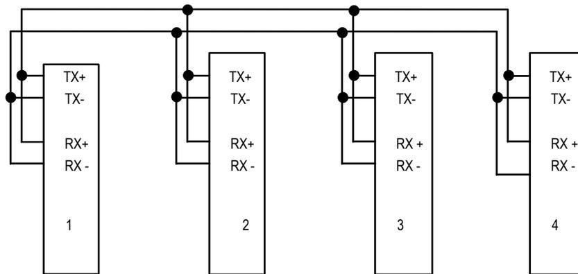
Note: The termination resistors from Station #2 and Station #3 have been removed.
